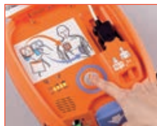
STEP 3 Push the shock button
